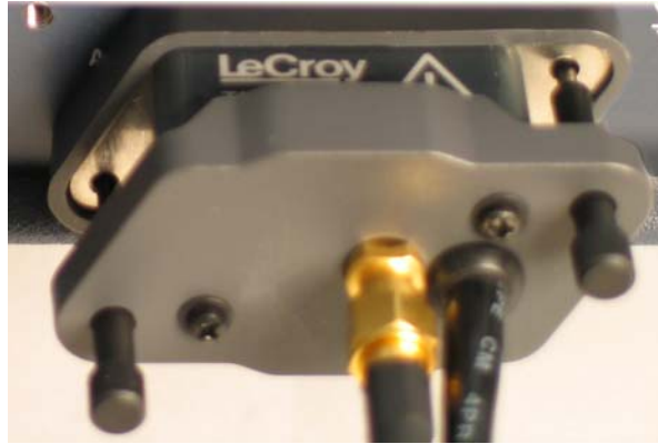
Connection of the TF-DSQ Fixture to the Scope Input
